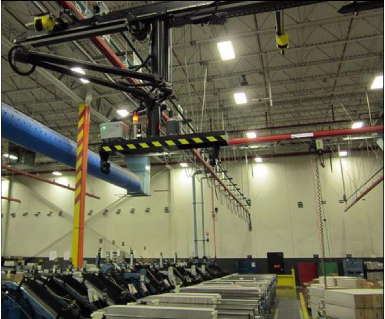
*Q-Track's RFID-based CANLOS system has been installed at a magazine printing company that uses automated cranes to move stacks of paper.*
